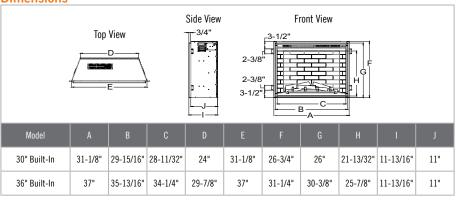
Dimensions above are in inches. Reference dimensions only. We recommend measuring individual units at installation. Refer to installation manual for detailed specifications on installing this product. SimpliFire reserves the right to update units periodically. Pictures in this brochure are not a true representation of the fireplace and/or flames.
